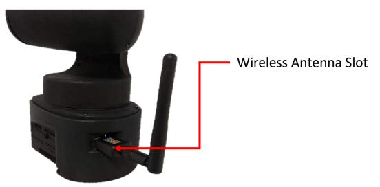
Reboot the device after inserting the antenna to enable internet connectivity.
